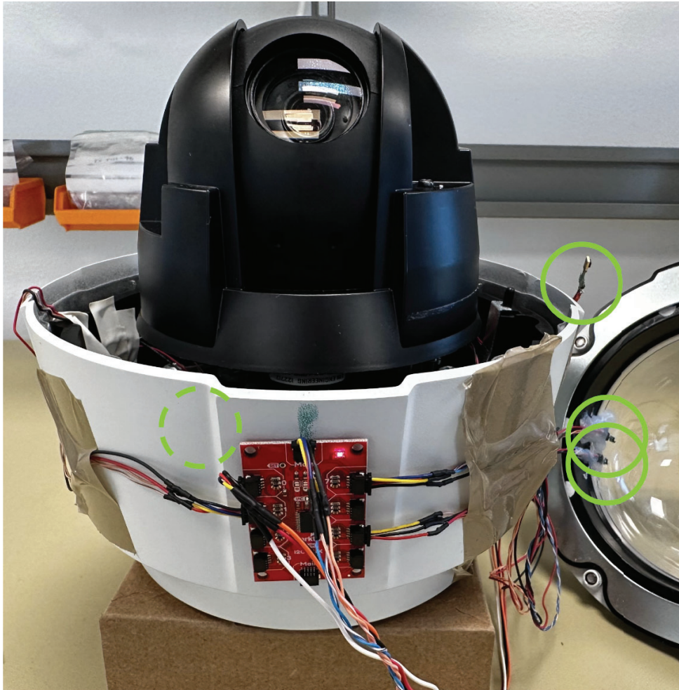
Figure 4.5: Image of the device under test with four SHT85 sensors. To make the sensor locations easier to identify, green circle markers have been added to the image.
