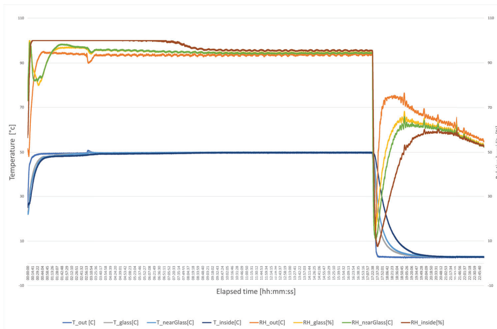
Figure 5.13: All the sensor inputs from test XI, the relative humidity and temperature from the four sensors.
