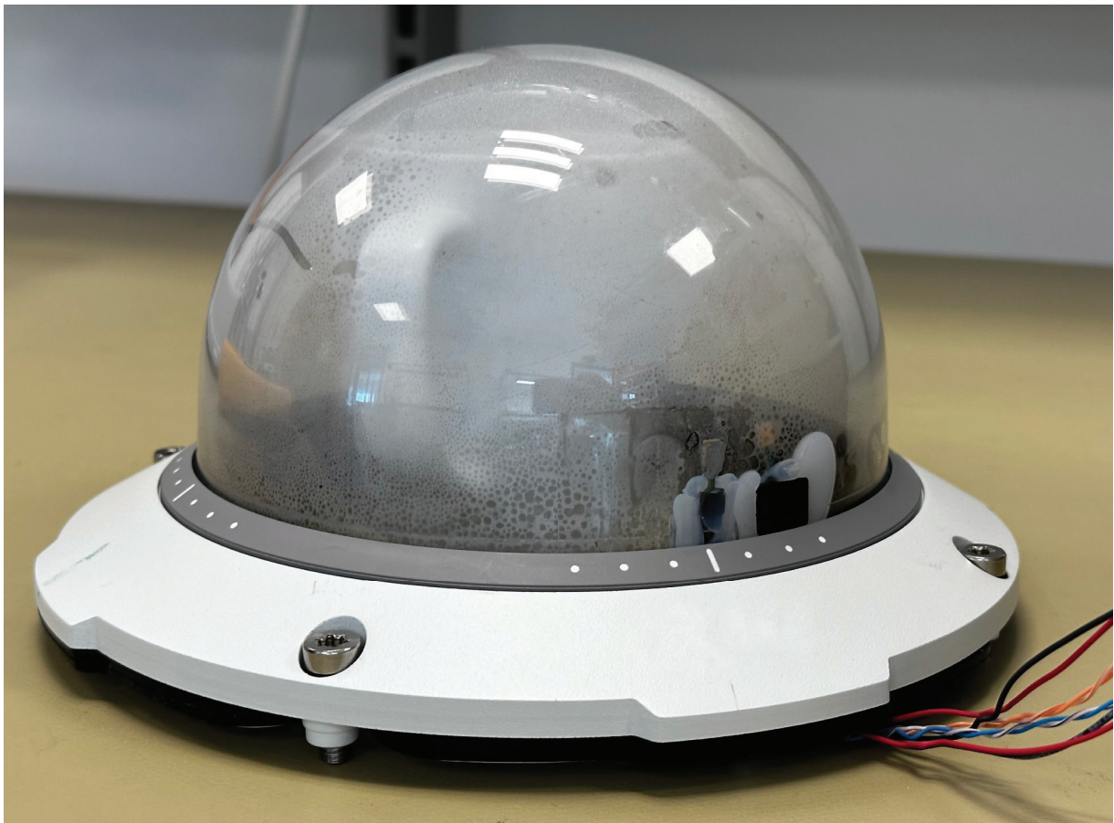
Figure 3.4: Test setup for testing of the hygrometer. The picture is taken during maximum fog presence.
